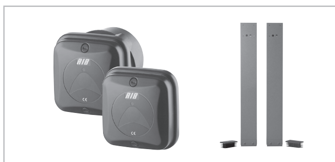
FIT SYNCRO PHOTOCELLS for the wall-installation code ACG8026 The range you can set is 10-20 m, 30÷60ft. You can fit many couples close together thanks to the synchronising circuit. Add the SYNCRO TRANSMITTER code ACG8028 for more than 2 photocells couples (up to 4). COUPLE OF BUILT-IN BOXES FOR THE FIT SYNCRO code ACG8051 PAIR OF COLUMNS FOR FIT SYNCRO H = 0,5 m code ACG8057
